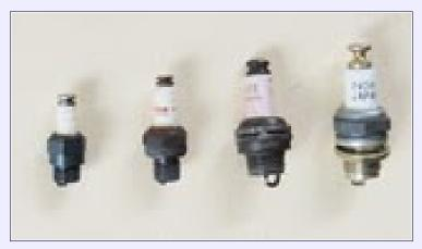
The spark plug, or "sparking plug", as the British charmingly prefer to call it, has an insulated electrode to which the coil high tension is connected by an insulated lead. As twenty thousand volts is nothing to be sneezed at, the high tension wiring and the spark plug deserve some respect. It will not, and cannot
