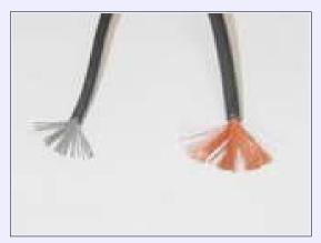
For the high-tension wire, you can't beat the sort of stuff used for electronic test equipment leads. Test-leads spend their entire life being bent, tugged, pulled, tied in knots, and stood on, while quite possibly being exposed to some rather inhospitable conditions. Accordingly, they are made with lots and lots of very, very fine strands about 0.001" in diameter. This makes the lead
