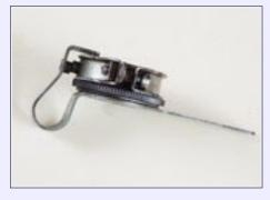
Generation of the high voltage which creates the ignition spark is initiated by the opening of the points. In almost all cases, the whole timer assembly can be rotated in relation to the cam allowing the position at which the contacts open in relation to top dead center (TDC) to be adjusted. This allows us to adjust the time at which the spark happens (hopefully) in relation to
